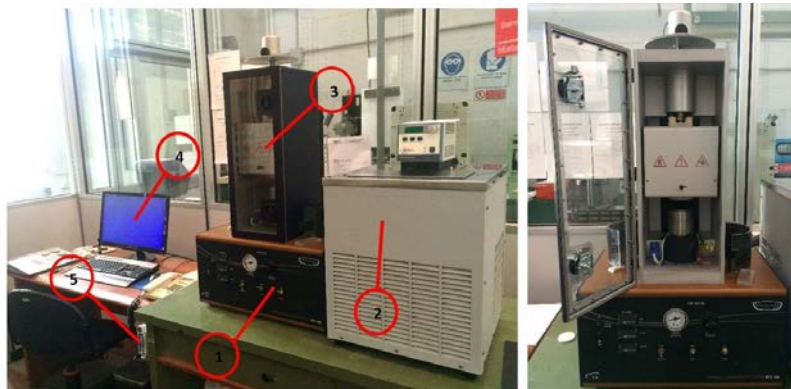
Figure 3. Thermo-physic measurement laboratory at CertiMaC, in Faenza. (1) Command and Control Panel in order to supervise the temperatures along the stack and the cylinder pressure. (2) Chiller with temperature automatic controller. (3) Stack section with HFM and Guard Heater. (4) Personal Computer with software and acquisition system. (5) Control and Command Panel for air and nitrogen system.
