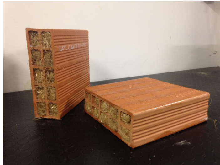
Figure 6. hollow bricks filled with hemp fibers.
