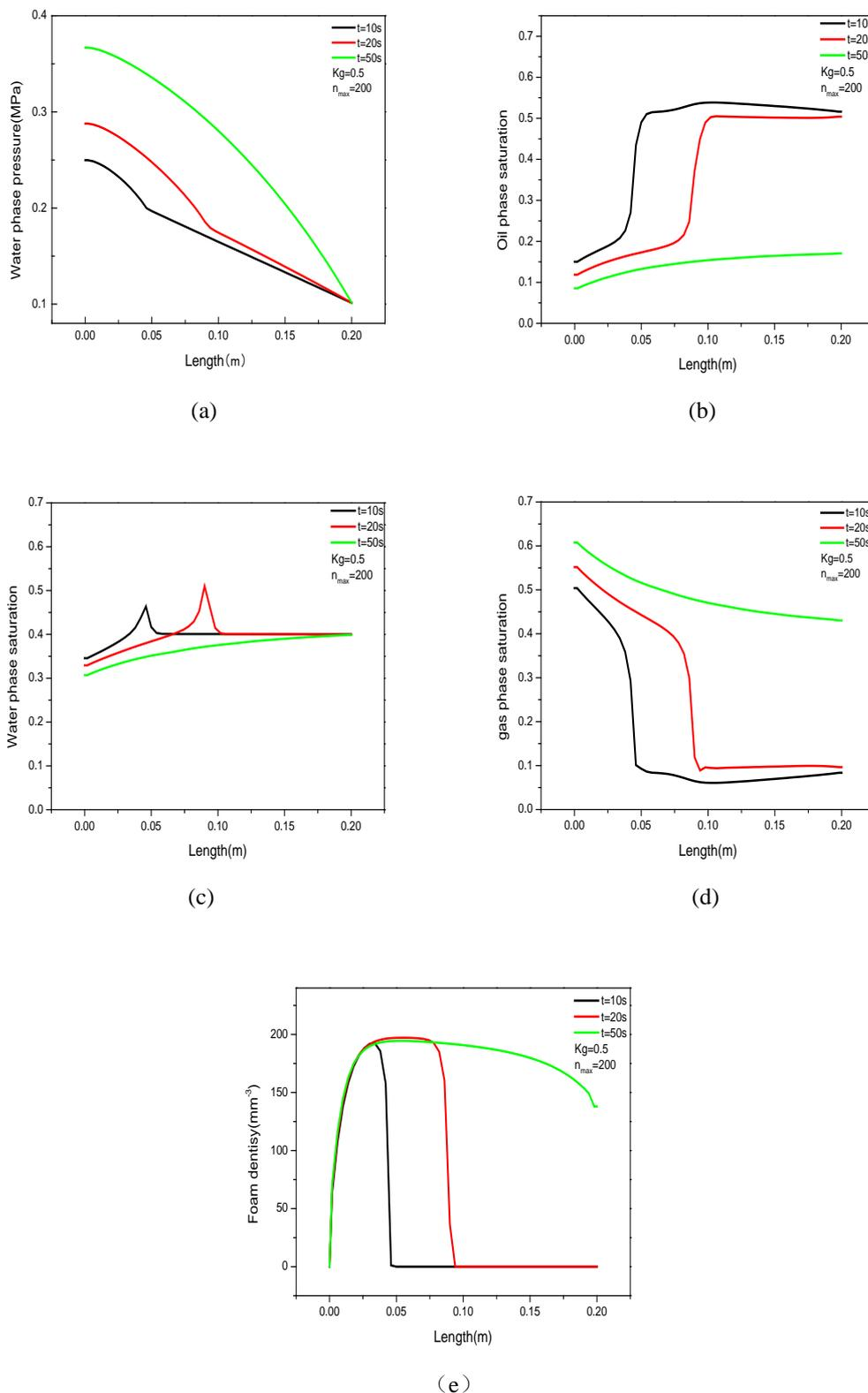
Fig.2 Different times of displacement (a) water phase pressure (b) oil phase saturation (c) water phase saturation (d) gas phase saturation (e) foam density along the course of change curve ( $Kg=0.5, n_{max}=200$ )
