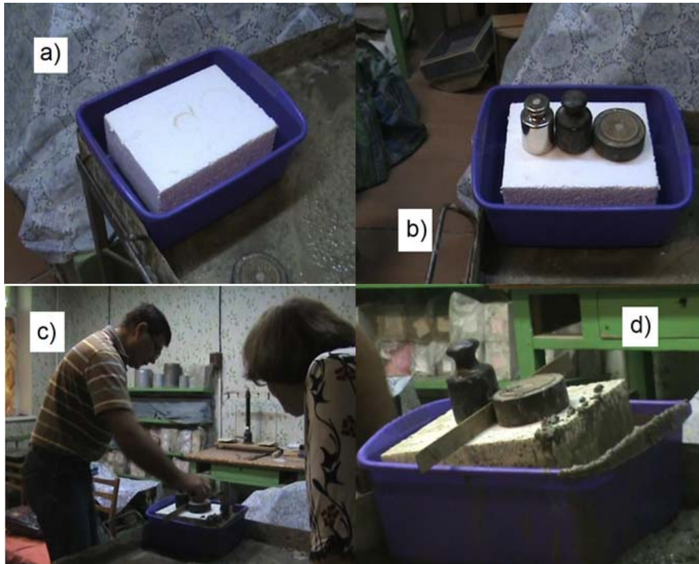
Fig.15 Experimental determination of insert floating-up force: a) foam polystyrene insert; b) insert cantledge; c) space filling with self-compacting concrete; d) insert floats up
