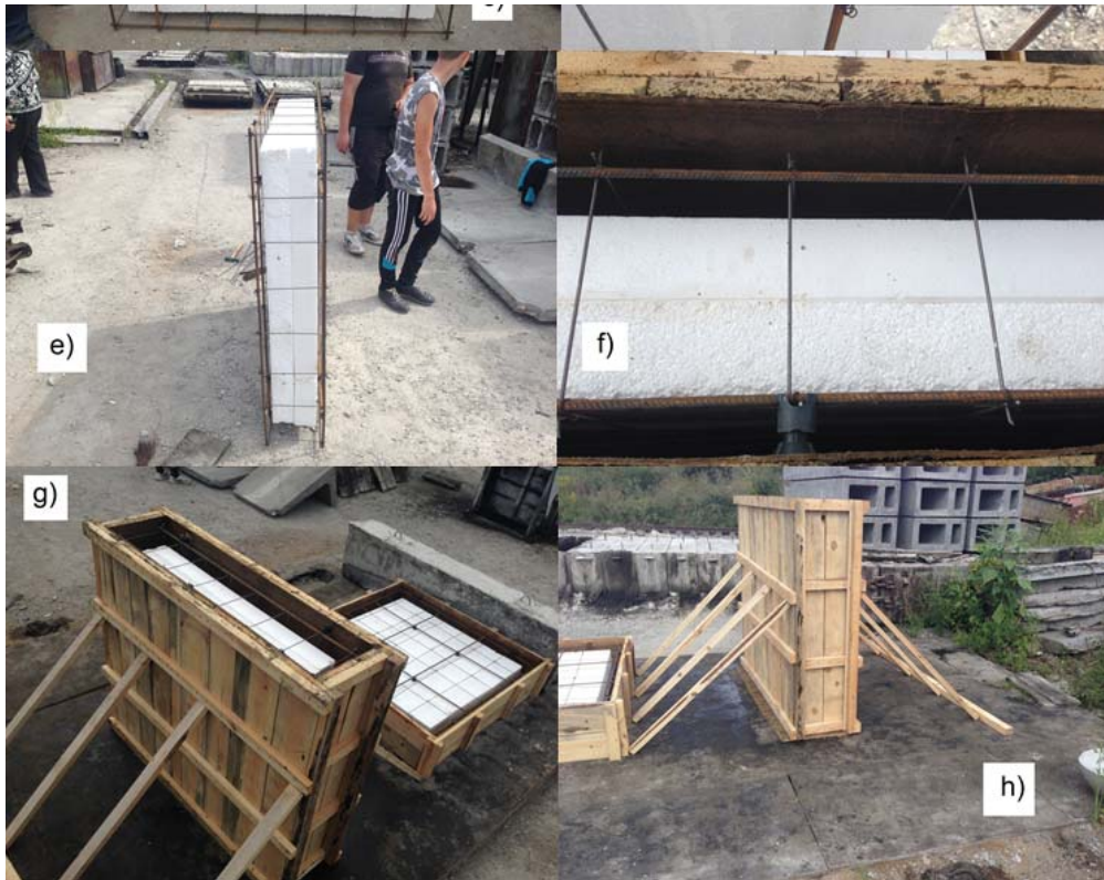
Fig.13 Concrete fabric and insert fixing process in manufacture of lightweight structure vertical elements: a) braces of vertical fabrics for maintaining insert in design position; b) vertical fabric design; c) insert fixation at four points; d) insert attachment to vertical fabrics; e) ready block consisting of concrete fabric and insert; f) chair ensuring thickness of protective layer for vertical fabric; g) top view of formwork for concreting; h) side view of formwork for concreting
