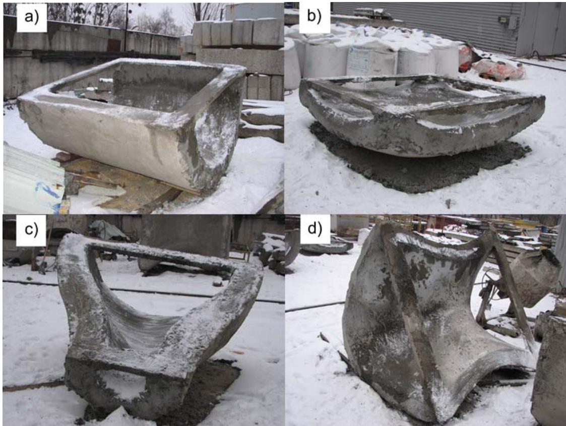
Fig.11 Cast reinforced concrete shells obtained by wet spraying: a) concreted cylinder fragment; b) concreted sphere fragment; c) concreted nodoid fragment; d) concreted hyperboloid fragment
