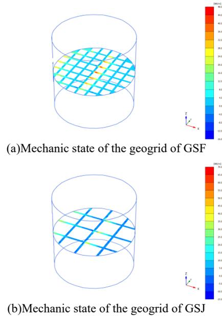
Fig. 11 Mechanical state of geogrid under different sizes
