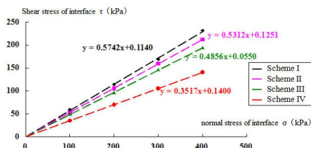
Fig. 5 Linear fitting of normal stress  $\sigma$  and shear stress  $\tau$  of the interface
