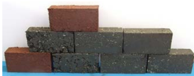
Figure 7. Freshly prepared clay-hemp bricks using L1 – GGBS, L2 – GGBS, and PC – GGBS mixtures
