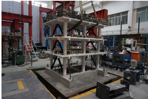
Fig.13 Specimen of shaking table test with reduced scale BRB
