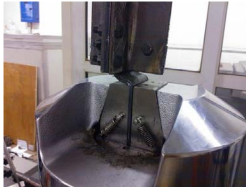
Fig.8 The buckling instability of testing specimen
