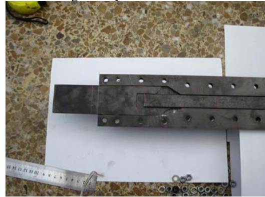
Fig.1 The core plate glues with additional plate Fig.2 Reserved gap for compressing of steel core
