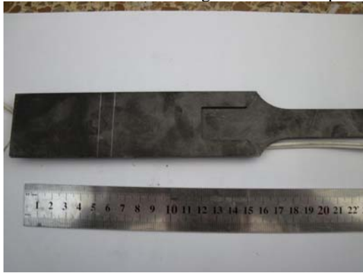
Fig.1 The core plate glues with additional plate Fig.2 Reserved gap for compressing of steel core
