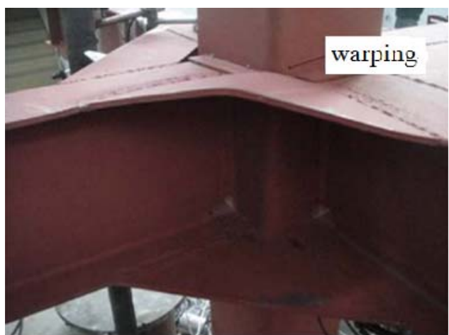
(a) Deformation of force-transforming plates in the experiment of ST-1
