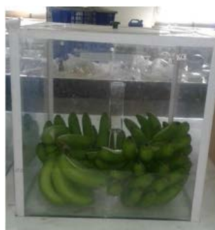
Plate 1. 1-MCP treatment chamber
