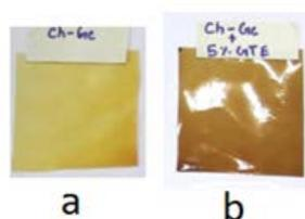
Fig 1. image of (a) Control film: ChGel and (b) active film: ChGel-GTE.
