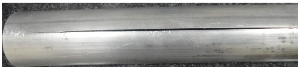
Fig. 1 Opening of port hole die extruded Al- 2.1 wt.% Mg tube along the seam.
