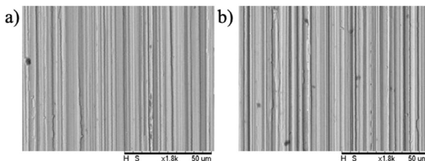
**Fig. 3.** Surfaces of VP Atlas steel after grinding with  $h_{eq}$ : (a) 0.07  $\mu\text{m}$  and (b) 0.14  $\mu\text{m}$ .
