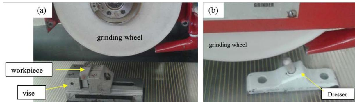
**Fig. 1.** Used setup (a) for the grinding tests and (b) for the dressing operation
