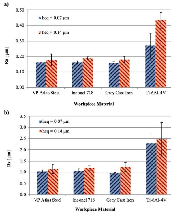
**Fig. 2.** Surface roughness versus equivalent chip thickness after grinding various metals. (a) Ra parameter. (b) Rz parameter.
