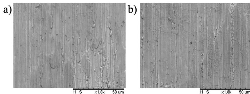
**Fig. 6.** Surfaces of the Ti-6Al-4V after grinding with  $h_{eq}$ : (a) 0.07  $\mu\text{m}$  and (b) 0.14  $\mu\text{m}$ .
