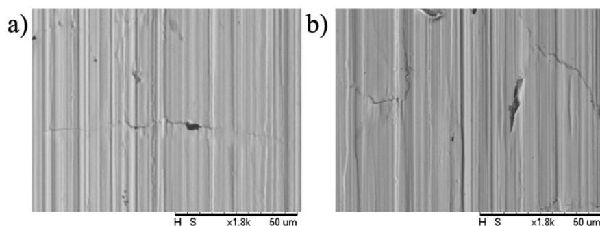
**Fig. 5.** Surfaces of the gray cast iron after grinding with  $h_{eq}$ : (a)  $0.07 \mu\text{m}$  and (b)  $0.14 \mu\text{m}$ .
