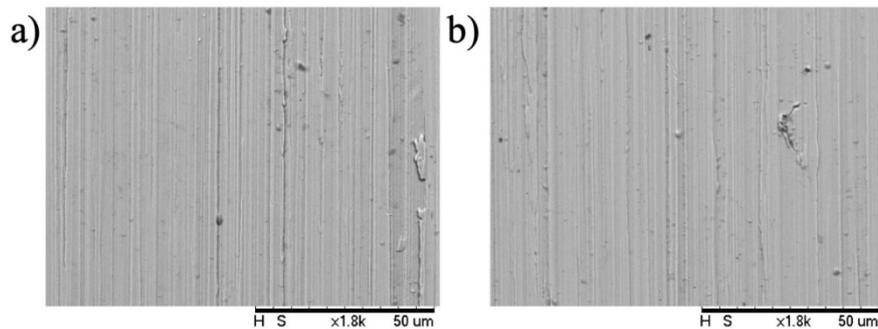
**Fig. 4.** Surfaces of the Inconel 718 after grinding with  $h_{eq}$ : (a)  $0.07 \mu\text{m}$  and (b)  $0.14 \mu\text{m}$ .
