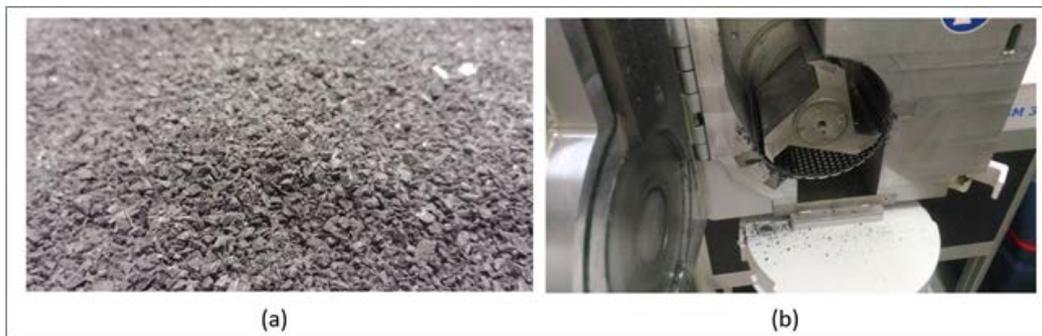
Figure 1. Grinded material (a) and a detail of the cutting mill RETSCH model SM300 (b).
