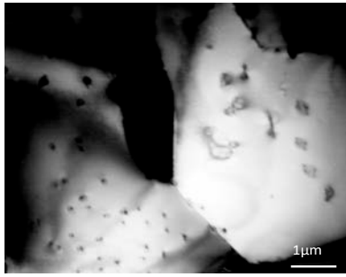
Figure 1. TEM bright field image of the as-received material showing the \alpha -Zr matrix.
