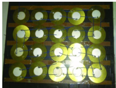
Fig. 2. Piezoelectric disks arrangements on power generation tile [13]
