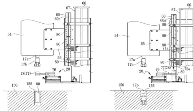
Figure 6. Mechanism for drilling and inserting SPC in concrete hole
