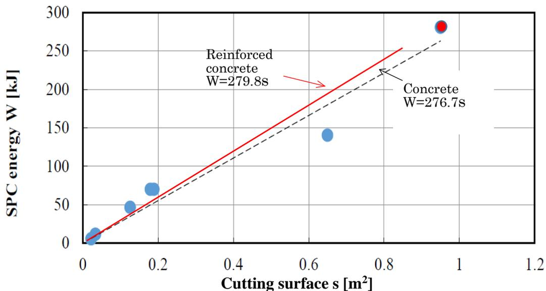
Figure 9. Relationship between amount of SPC energy and cutting surface area
