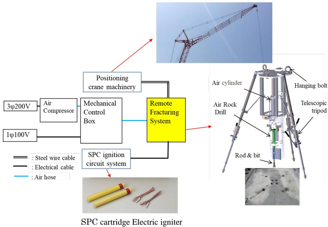
Figure 3. Total design of Remote-Control Cracking System by SPC
