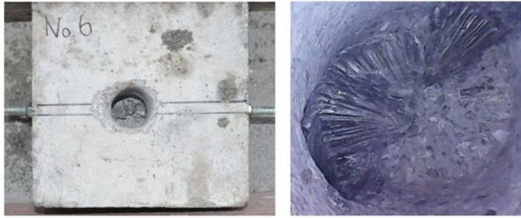
Figure 5. Steel bar which was cut by the concrete bit
