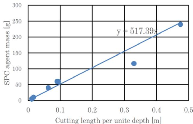
Figure 11. Relationship between SPC mass  $y$  and crack length  $x$  per unit depth.
