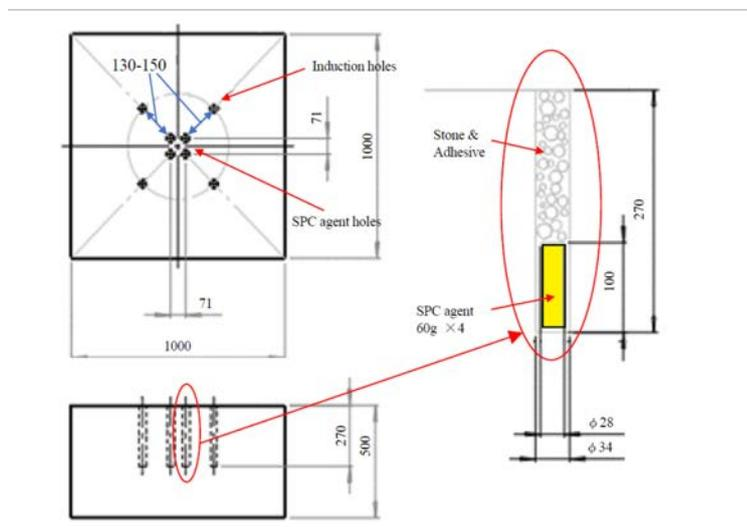
Figure 7. SPC cartridge inserting to hole and close by glue
