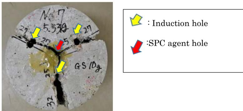
Figure 2. Controlled cracking of a small concrete piece by the SPC agent [4].
