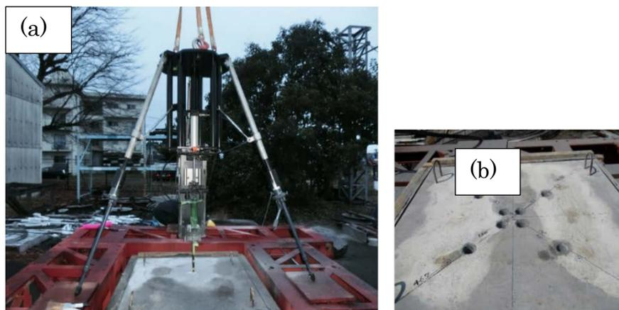
Figure 4. (a) Setting of Remote Cutting System and (b) boring test of reinforced concrete
