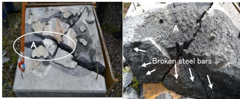
Figure 8. Cracked concrete and steel bars cut by SPC on concrete surface
