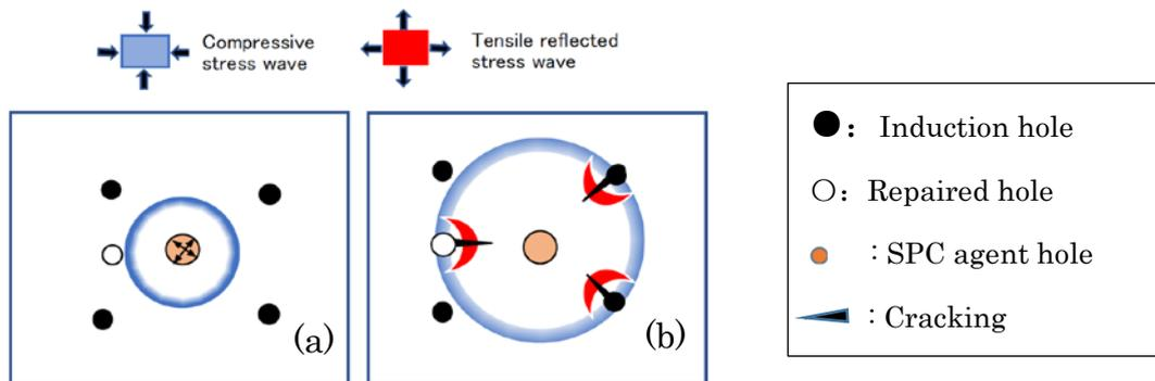
Figure A-1. Schematic illustration of tested concrete, indicating SPC agent, induction hole, and repaired hole. The elastic wave initiates from SPC in Figure A-1(a) and reflect at induction hole Figure A-1(b). Areas of compressive stress are shown in blue, and red areas represent tensile stress.
