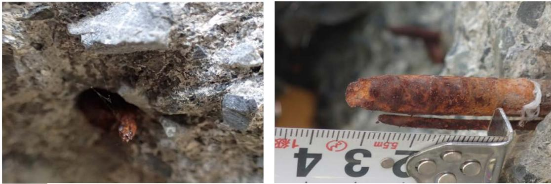
Figure 10 Broken steel bar surface with low energy by high-speed tensile condition
