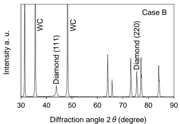
Figure 6. XRD patterns of the synthesized diamond film for Case B.
