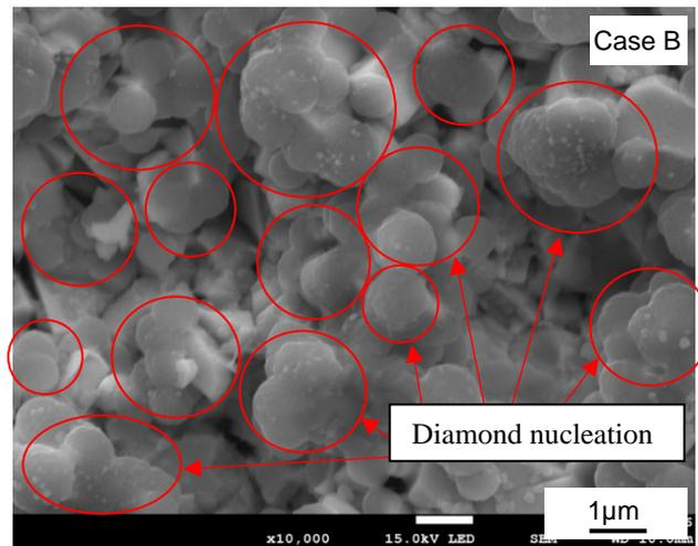
Figures 11. SEM image of the substrate surfaces of the synthesized films after the first 60 s for Case B.
