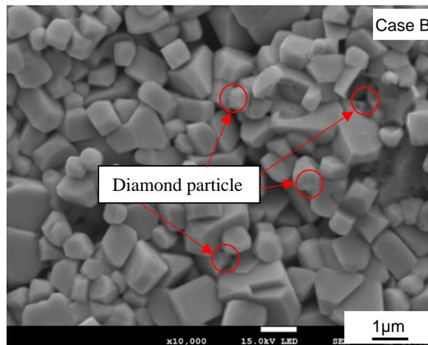
Figures 15. SEM image of the substrate surface after seeding treatment for Case B.
