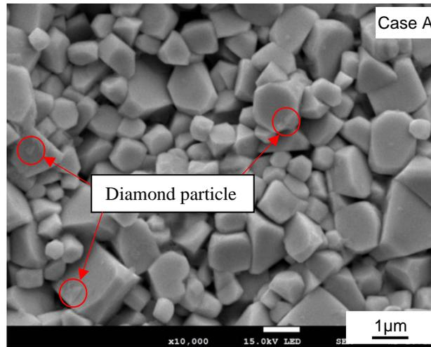
Figures 14. SEM image of the substrate surface after seeding treatment for Case A.
