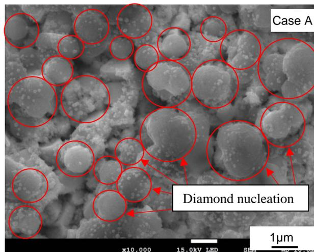
Figures 10. SEM image of the substrate surfaces of the synthesized films after the first 60 s for Case A.
