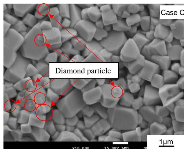
Figures 16. SEM image of the substrate surface after seeding treatment for Case C.
