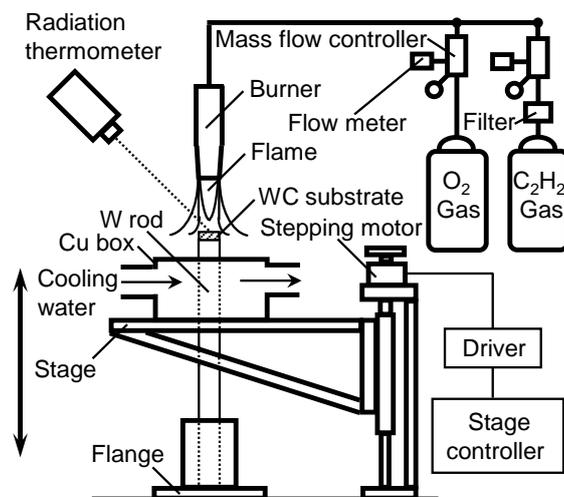
Figure 1. Experimental setup for synthesizing diamond film by acetylene-oxygen flame combustion.
