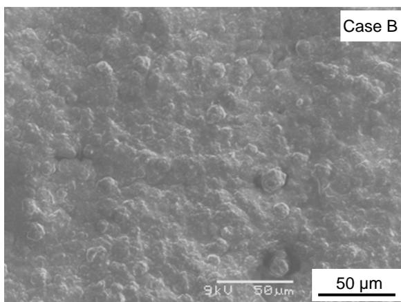
Figure 5. SEM image of the synthesized diamond film for Case B.
