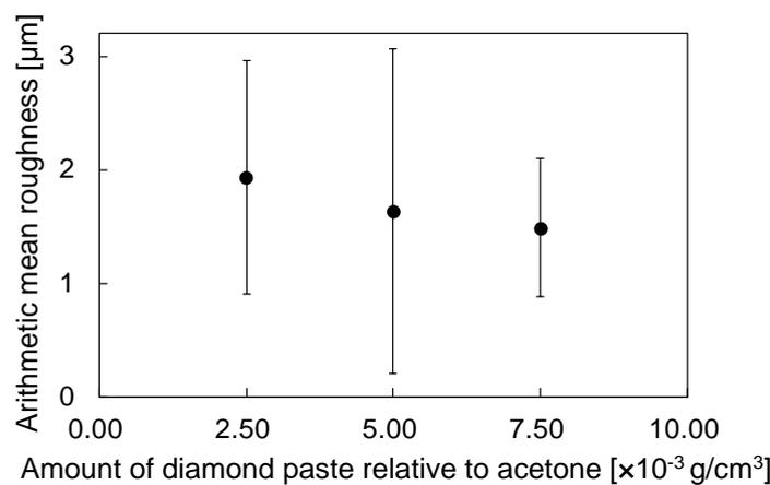
Figure 9. Results of surface roughness of synthesized diamond films on WC substrates for each case.
