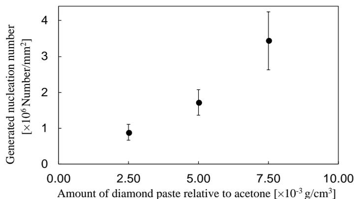
Figure 13. Results of measuring the number of particles nucleated on the substrate after 60 s of synthesis for each case.
