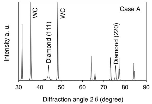
Figure 4. XRD patterns of the synthesized diamond film for Case A.
