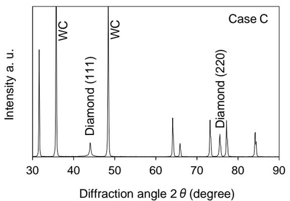
Figure 8. XRD patterns of the synthesized diamond film for Case C.
