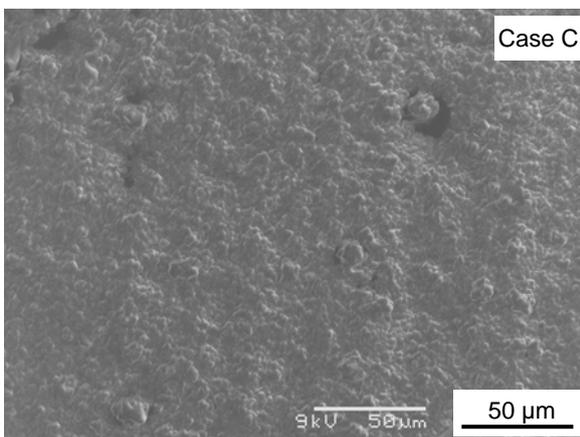
Figure 7. SEM image of the synthesized diamond film for Case C.
