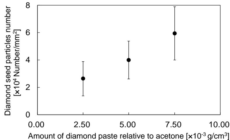
Figure 17. The results of the number of particles after seeding treatment for each case.
