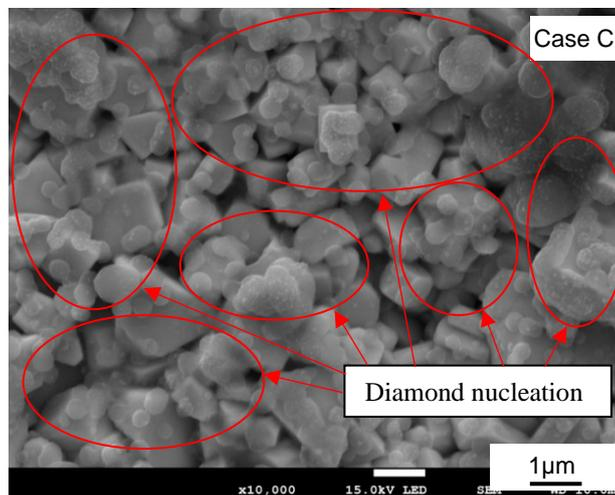
Figures 12. SEM image of the substrate surfaces of the synthesized films after the first 60 s for Case C.
