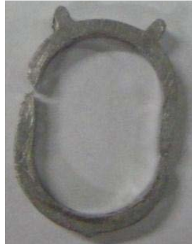
Fig. 2a Typical 3 mm wide ring tensile testing sample Fig. 2b Typical ring tested sample
