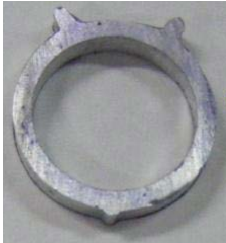
Fig. 2a Typical 3 mm wide ring tensile testing sample Fig. 2b Typical ring tested sample
