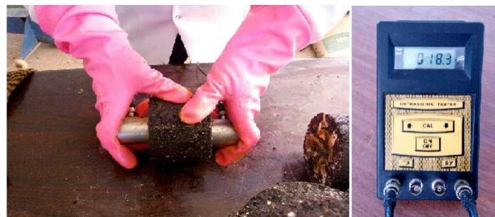
Figure 3. Ultrasonic pulse velocity Measurement in process
