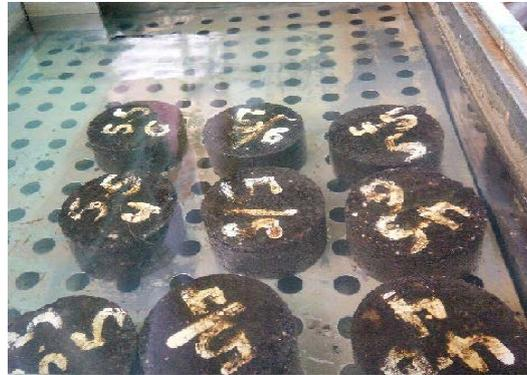
Figure 4. Specimens Under Moisture Damage Process
