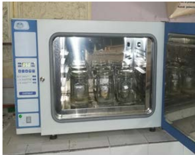
FIGURE 2. Experimental apparatus for the sorption isotherms measurement
