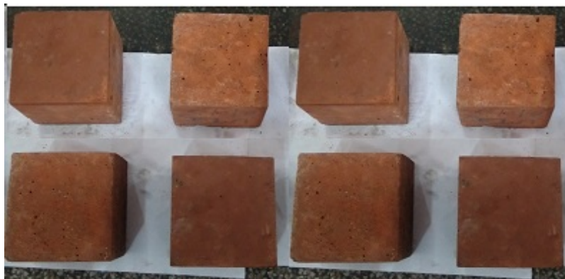
Fig 3. Cubic samples (70x70x70 mm) prepared in this study
