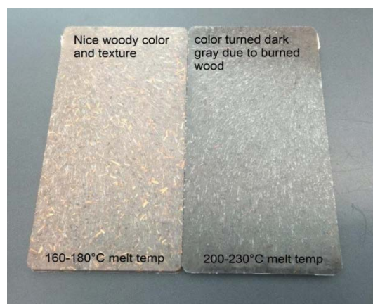
Figure 3. Effect of processing temperature on the degradation behavior date palm fiber
