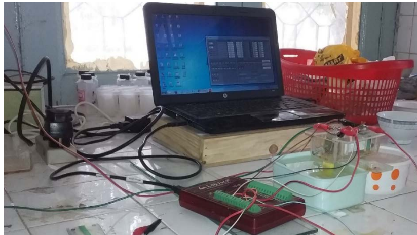
Fig 2. The whole setup of electrokinetic desalination
