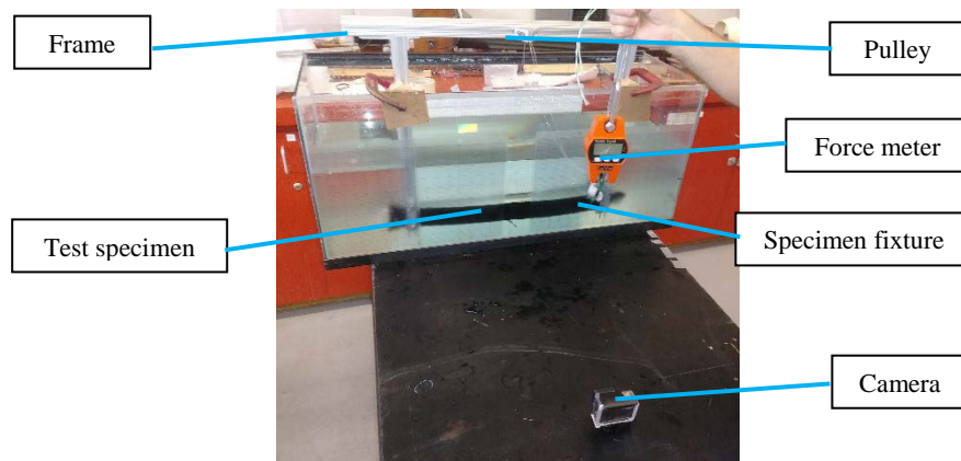
Figure 4. Beam bending test setup
