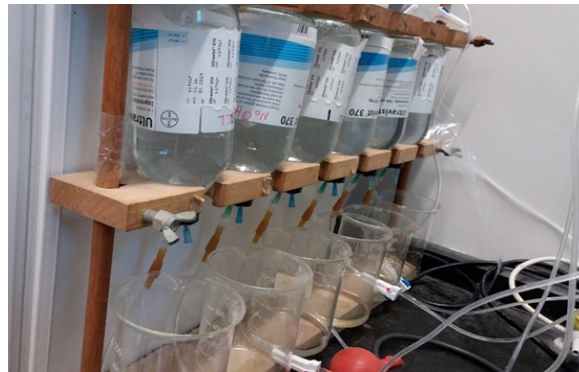
Figure 4. Biogas measurement unit
