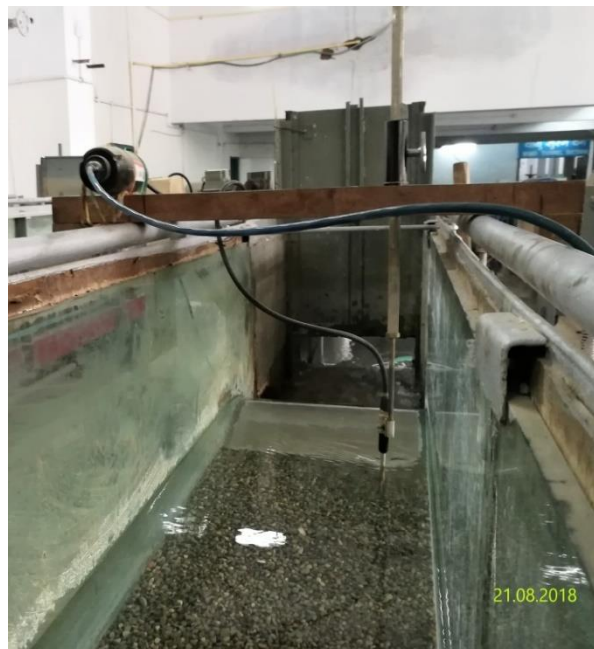
Figure 1. Setup with Acoustic Doppler Velocimeter
