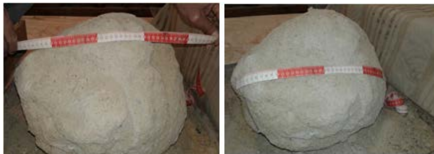
Fig. 5. Bottom block after cementation.
