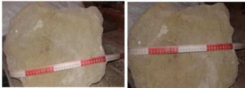
Fig. 4. Surface block after cementation.
