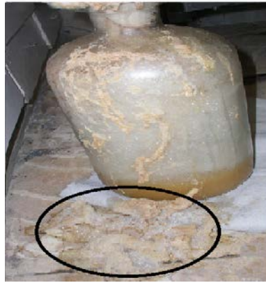
Fig. 2. Overflow of bacteria out of the container due to the excess presence of air
