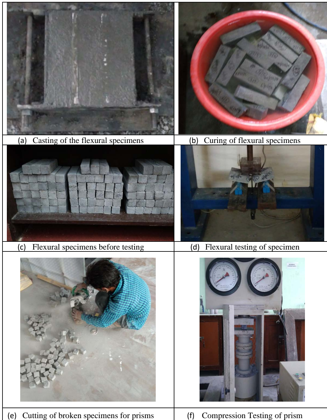
Fig. 3. Various stages of casting and testing
