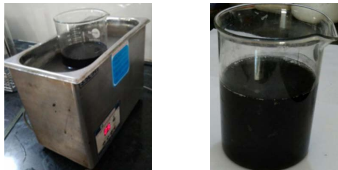
(c) Sonication for dispersion of MWCNT (d) Sonicated water after 30 minutes of sonication
