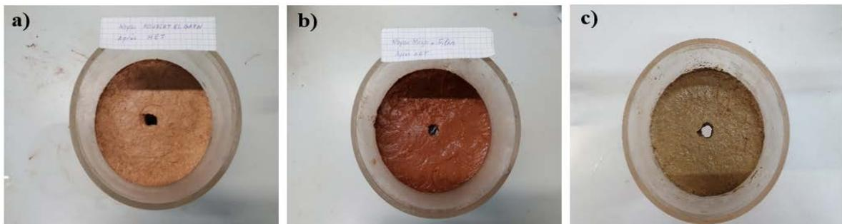
Fig. 9. Pictures of the hole after HET test of core soils using cell N°1 from (a) Koudiat El Garn dam, (b) Mazer dam, and (c) Moulay Boucheta dam
