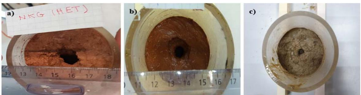
Fig. 10. Pictures of the hole after HET test of core soils using cell N°1 from (a) Koudiat El Garn dam, (b) Mazer dam, and (c) Moulay Boucheta dam
