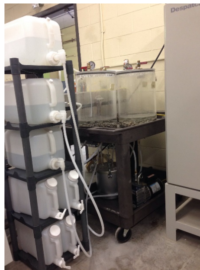
Figure 1. Vacuum impregnation of rest set-up for recycled concrete aggregate
