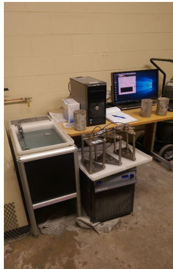
Figure 2. AFTC2 CTE Measurement System
