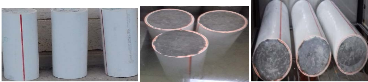
Fig. 1 CFPT specimens cured in (a) open air; (b) water; (c) sealed.
