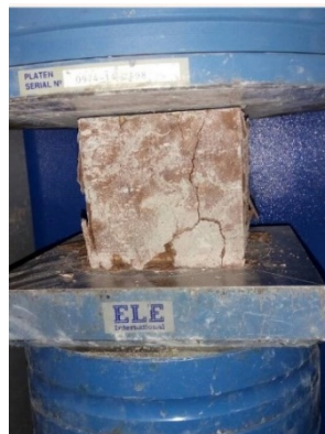
Figure 4. Typical cube specimen failure of colored concrete under the compressive strength test.
