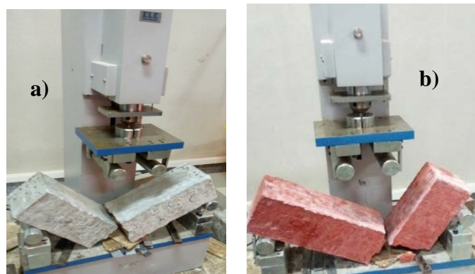
Figure 5. Flexural prisms while splitting into two pieces as subjected to four-point loading for (a) green pigmented prism specimens and (b) red-pigmented prism specimens.
