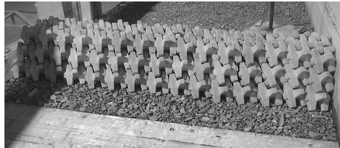
Figure 2. A photograph of a detached breakwater built by stacking the wave dissipating block models in three layers. In each row along the onshore x -axis direction, six, five, and four blocks were arranged in the bottom, middle, and top layers, respectively. In each row along the y -axis direction, 15 blocks were arranged.
