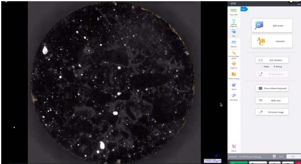
Figure 16. Screenshot of VHX Software User Window with a Fully Stitched Concrete Sample.
