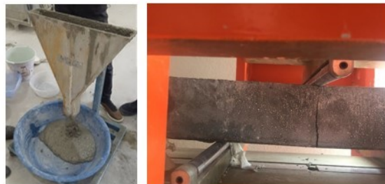
Figure 3. V-funnel test in self-compacting concrete and bending test
