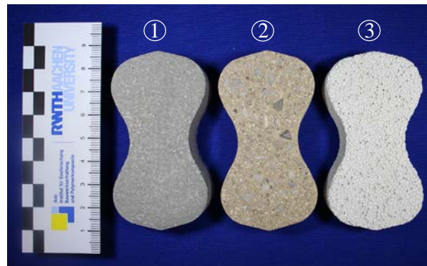
Figure 6. Bone-shaped briquet specimens of the three materials (exemplarily): (1) RM-A4, (2) PM21, (3) ACC2-350
