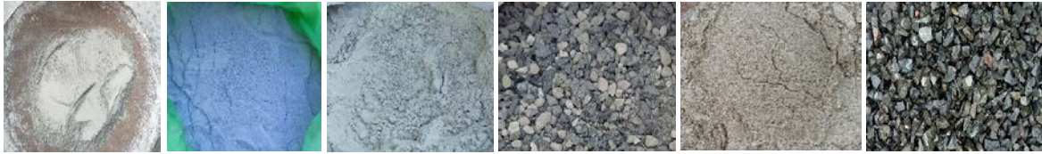
Fig. 1. Used materials for the preparation of the specimens (from left: cement, silica fume, fly ash, steel slag, sand, stone chips)
