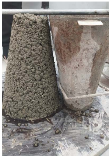
Figure 3. Slump to test workability
