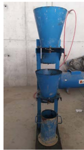
Figure 4. Compacting factor testing
