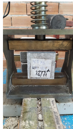
Figure 6. Strength of cube by tension
