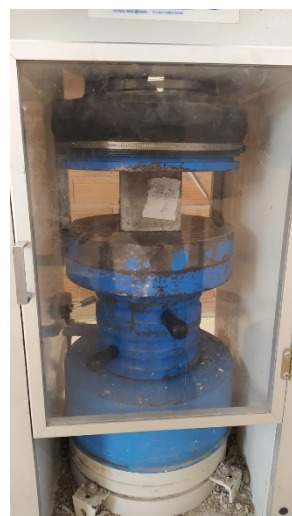
Figure 5. Cube strength by compression
