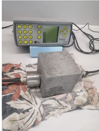
Figure 7. Pulse velocity on concrete sample
