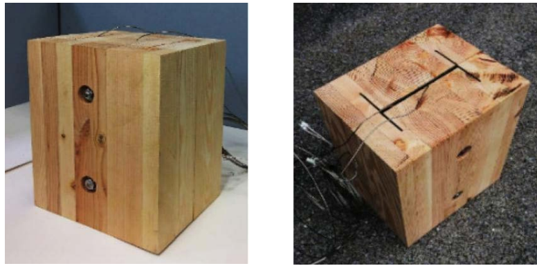
Figure 2. Schematic diagrams of the CST column specimen under fire in the laboratory [14]
