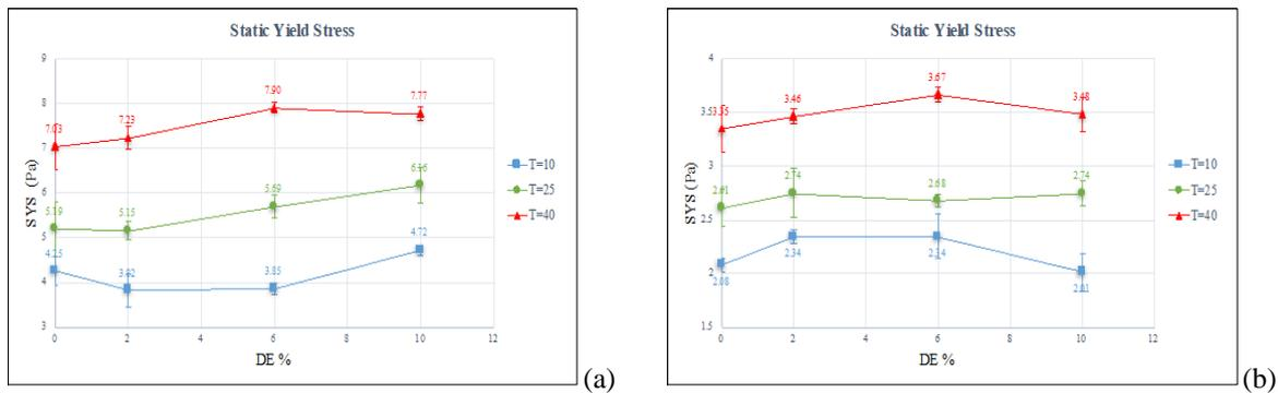
Fig. 13. Static yield stress from protocol 2 against DE replacement level (a) w/b=0.5 (b) w/b=0.6
