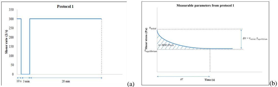
Fig. 2. Protocol 1 (a) Testing procedure (b) Measurable parameters
