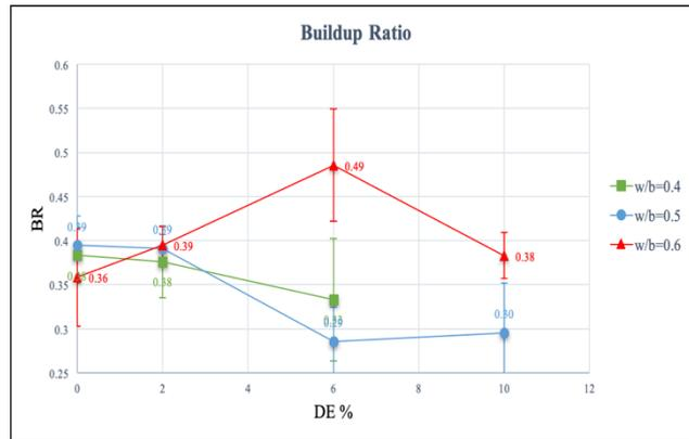
Fig. 10. Build-up ratios from protocol 3 against DE replacement levels
