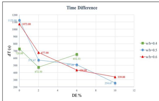
Fig. 8. Time to reach to steady state against DE replacement level for protocol 1
