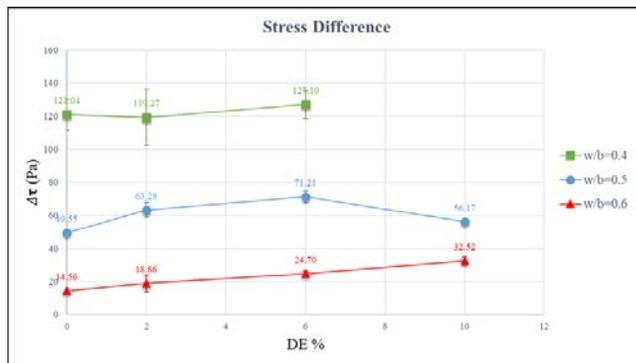
Fig. 7. Drop in shear stress against DE replacement level for protocol 1
