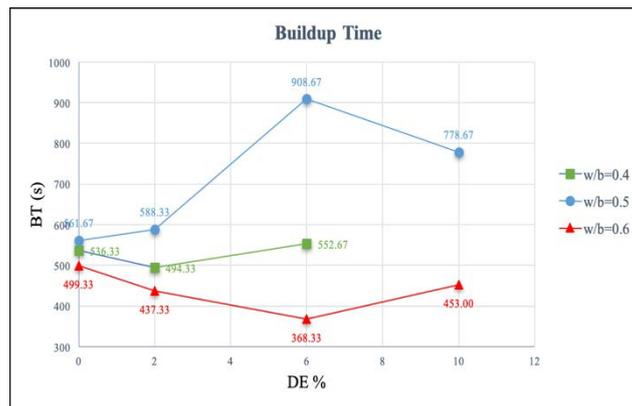
Fig. 11. Build-up time from protocol 3 against DE replacement levels
