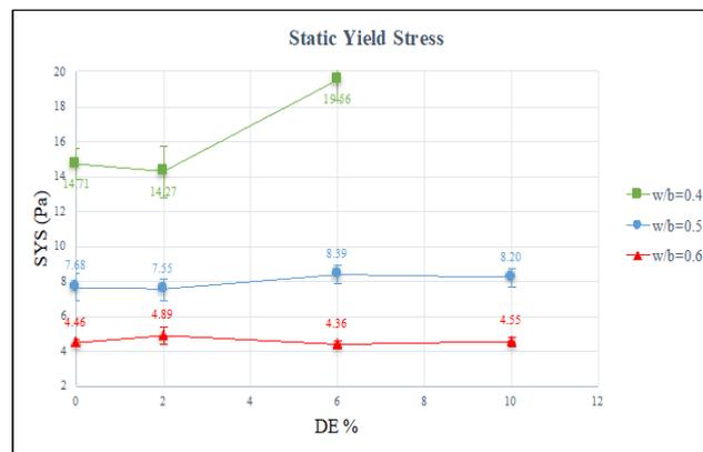
Fig. 9. Static yield stress against DE content from protocol 2
