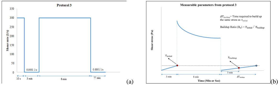
Fig. 4. Protocol 3 (a) Testing procedure (b) Measurable parameters
