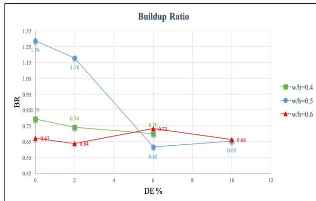
Fig. 12. Build-up ratios from protocol 4 against DE replacement levels
