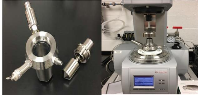
Fig. 1. Pressure cell and magnetic coupling
