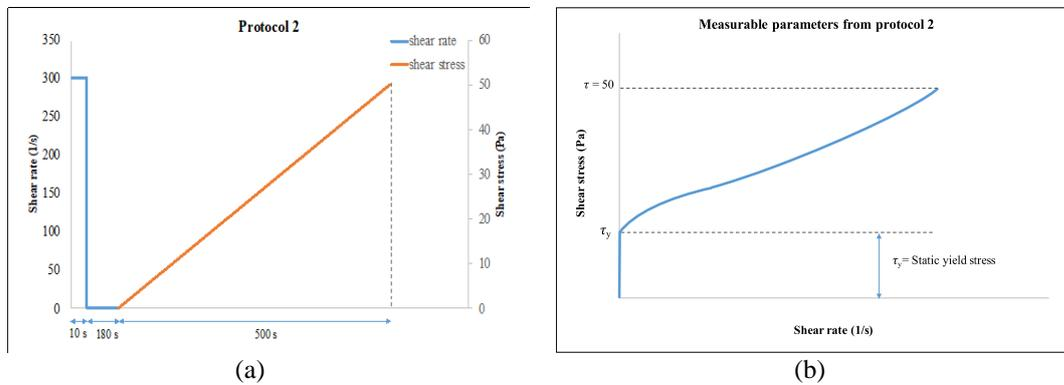
Fig. 3. Protocol 2 (a) Testing procedure (b) Measurable parameters
