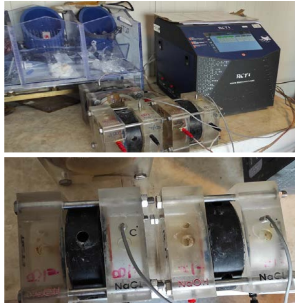
Figure 7. Chloride ion penetration measuring device
