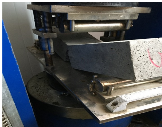
Figure 3. Flexural strength device
