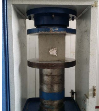
Figure 2. Compressive strength device
