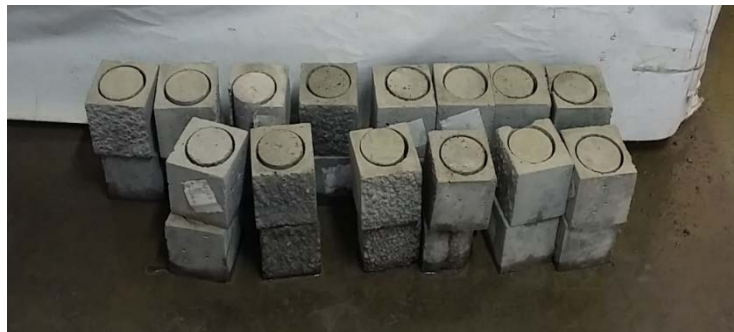
Figure 5. Preparing samples for water absorption test
