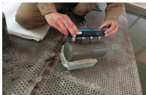
Figure 6. Electrical resistivity test
