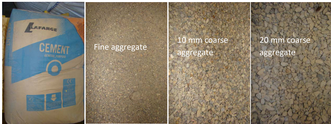
Figure 1. cement and aggregates used for concrete specimens
