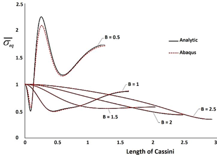
Figure 5. Dimensionless equivalent stress in the shells of the Cassini head
