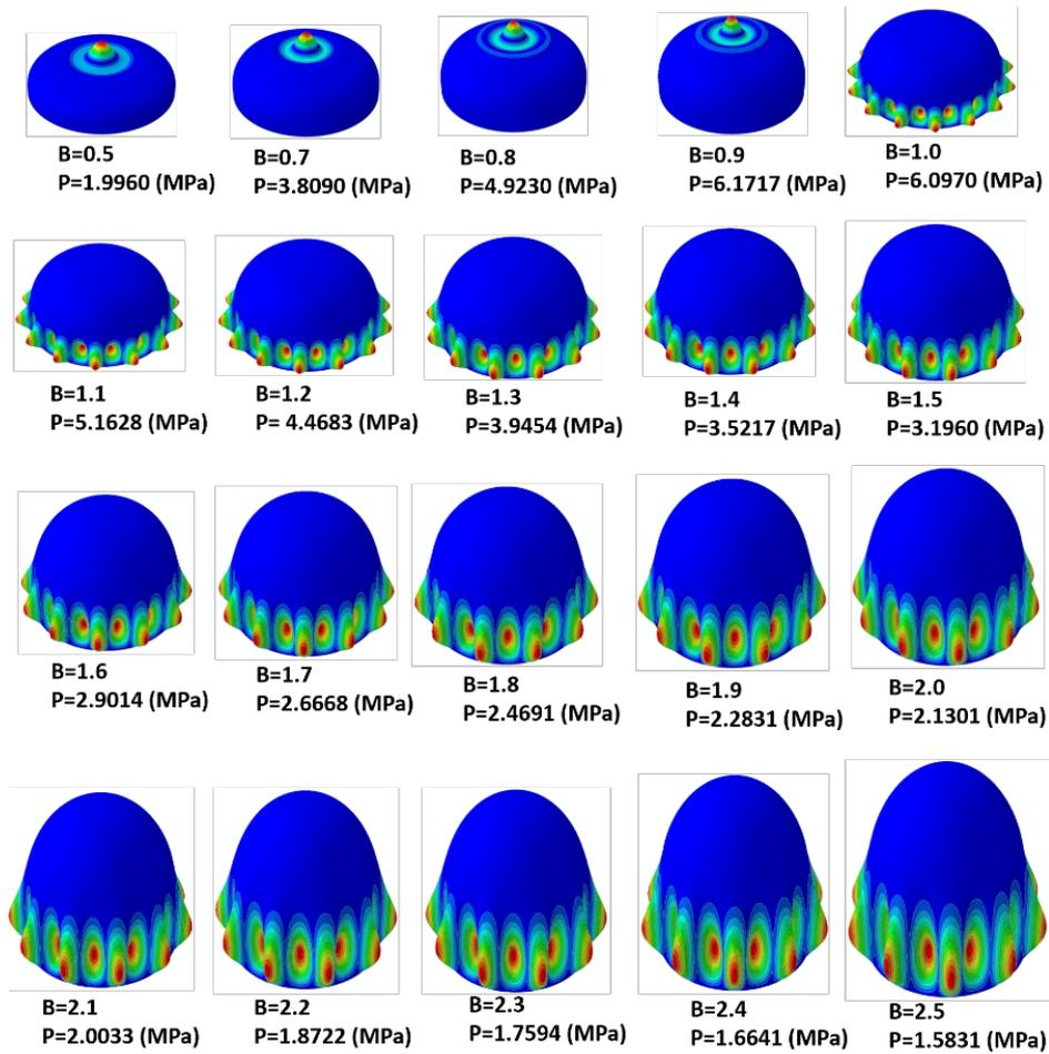
Figure 7. First mode shape of Cassini shells with different shape parameters
