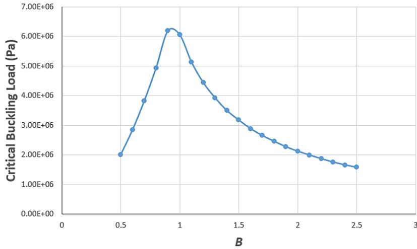
Figure 6. Critical load of linear buckling of Cassini heads
