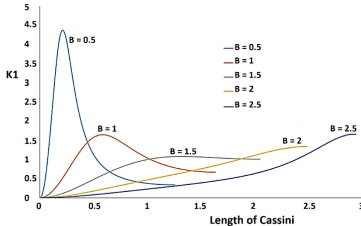
Figure 4. Generative curvature in the shells of the Cassini head
