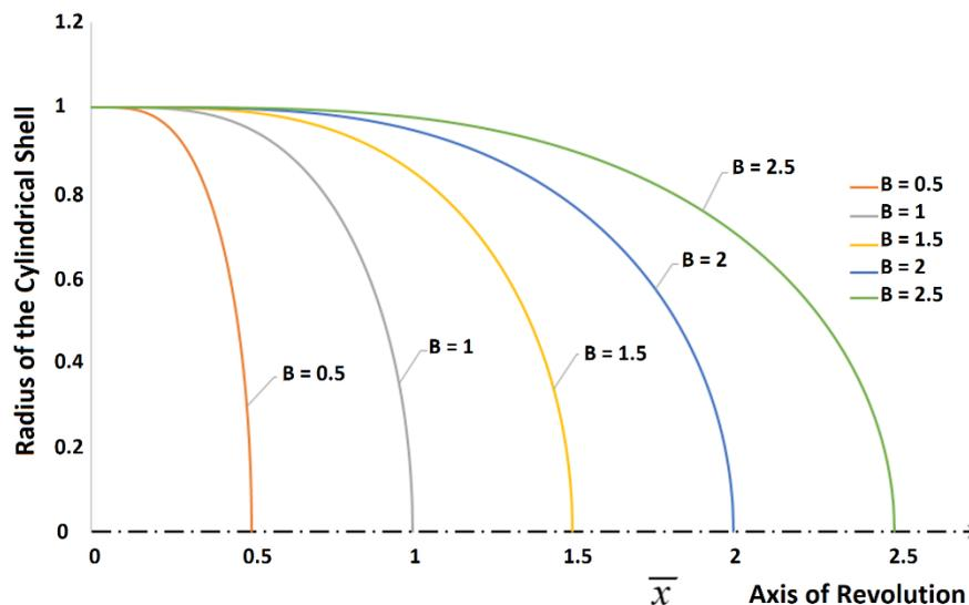
Figure 1. Cassini ovaloidal heads with different shape parameters
