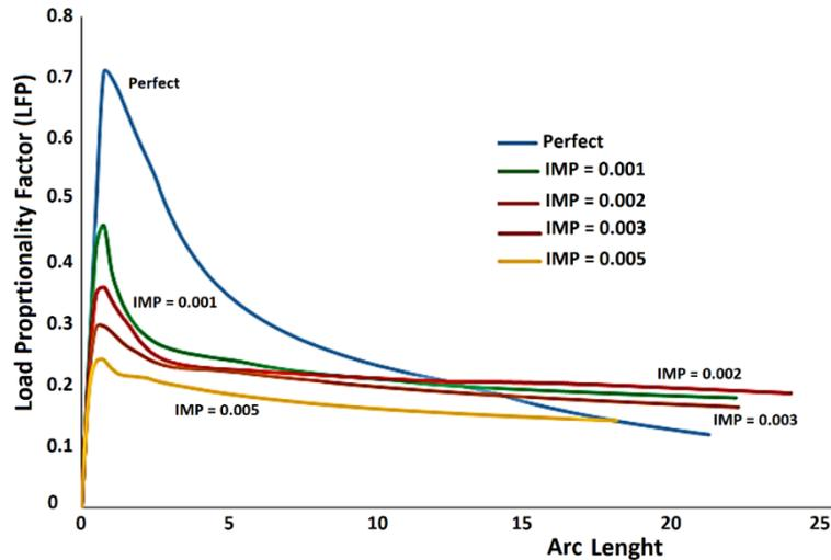
Figure 8. LPF diagram of Cassini's head with different geometric shape defects
