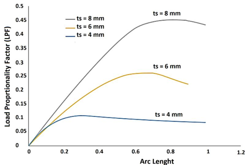
Figure 9. Effect of thickness on post-buckling behavior of Cassini head (imp=0.001)
