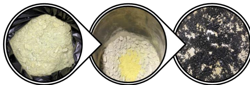
Fig 2. Using NMF Particles in Dry Mixing Process
