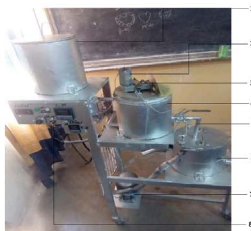
Figure 1. Invented 3-Stage Recycling Batch Pasteurizer for raw-milk (1-Hot water storage tank, 2- Water pump, 3- Stirrer, 4- Pasteurization tank, 5- 20 mm Aluminum pipe, 6- Cooling tank, 7- Frame, 8- Control panel)
